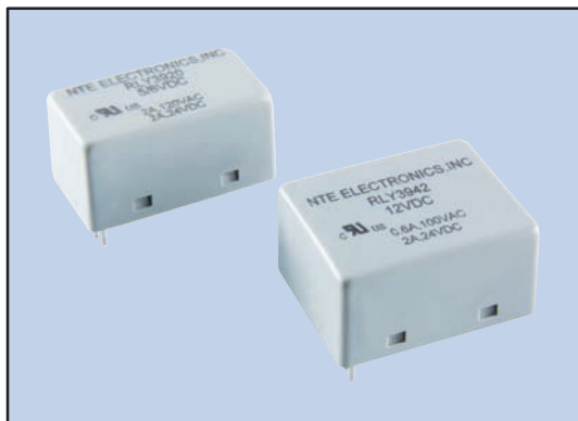
SPDT, 1 Form "C" (Bottom View)
