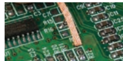
Match braid width to contact area
