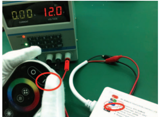
4. Touch the Power On button within 3 seconds and the receiver's indicator will turn blue. You have now successfully programmed both your remote and receiver.
