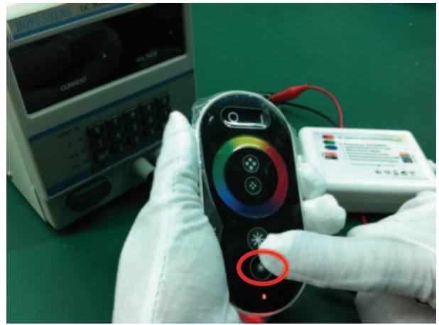
2. Touch the brightness-decrease button to initiate programming
