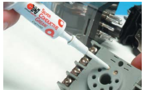
Step 3.2: Apply conductive grease to connectors
