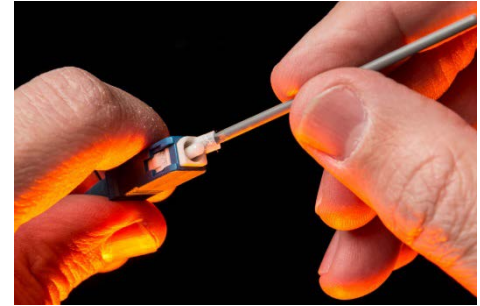
Step 5.3: Clean barrel of ceramic ferrule with swab
