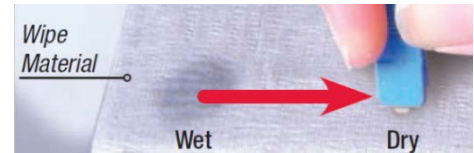
Step 5.2: Clean fiber optic end-face with Combination Cleaning™ process
