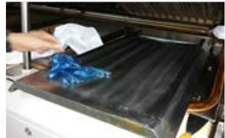
Coating easily peels-off
