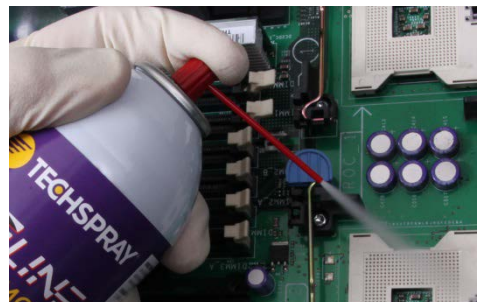
Step 1.2: Remove moisture with E-LINE™ IPA cleaner and Vortex™ Duster
